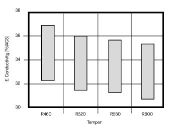
Electrical conductivity is strongly influenced by cemical composition A high level cold deformation and small grain size decrease the electrical conductivity moderately. Minimum conductivity level can be specified.
