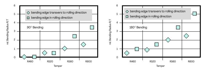
Tending test according to EN ISO 7438 is done with 10 mm wide samples. Smaller samples in general - as well as lower thickness - allow a lower bending radius without cracks. If needed we supply bending optimized temper classes that far exceed standard quality. Please take care when comparing with ASTM E290 results, there the bend definition direction is contradictory.
